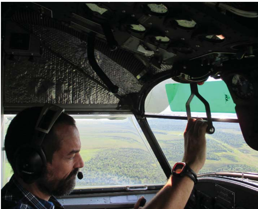
The author at the controls fine-tuning the engines to get them synchronised. Note that the throttles are on the roof panel. Pitch levers can be seen aft of the throttles.
