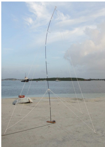
The famous cabin-baggage antenna, this time at PJ7/ZS6EZ on Sint Maarten.
